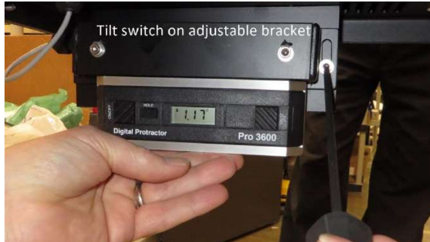
Figure 15: Tilt switch bracket detail
