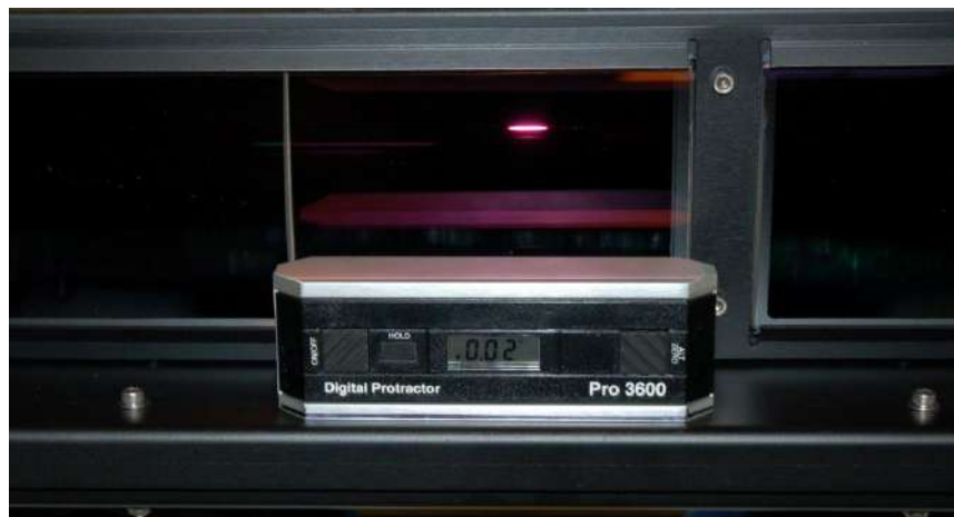
Figure 13: LHA with the digital inclinometer in place
